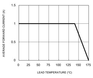
Fig.1 Forward Current Derating Curve
